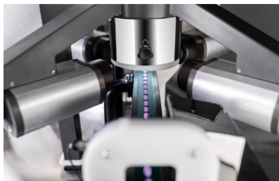
Img 2: Netra VS6 Camera setup
